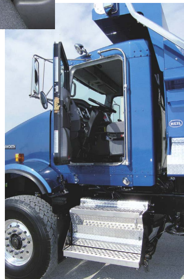
The cab sits 3.5 inches higher than on other T800s, so each step's a legful. But grab handles outside and inside help.
