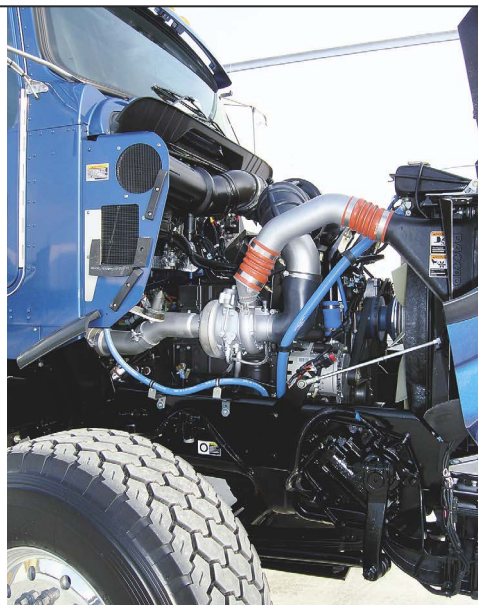
The Cummins ISL grows nicely and makes good power. It has no EGR and won't until 2007.
