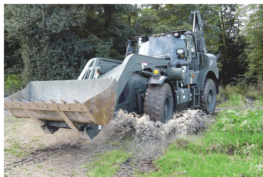
G.I. Joe's new backhoe rolls with full suspension and anti-lock brakes. It can lift 2 tons and dig about 13 feet deep.
