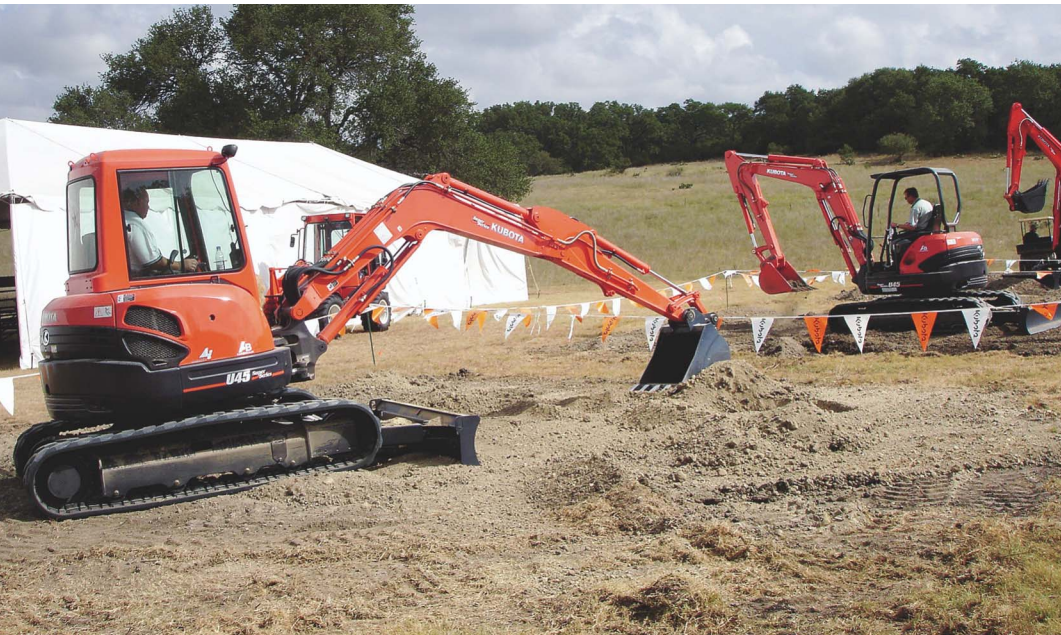
Kubota's Super Series U45 mini-excavator, seen here at its introduction to Kubota dealers this fall, features a climate-controlled cab, deluxe suspension seat and two-pattern-control selection.
