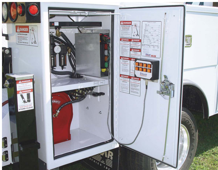
Stellar Industries' new control panel can be mounted in various convenient locations in the truck, and more than one panel can be used — for example, one on the crane-compartment door (shown here) and another in the cab. The panel has a provision for optional pre-wired switches (with up to 20-amp capability).
