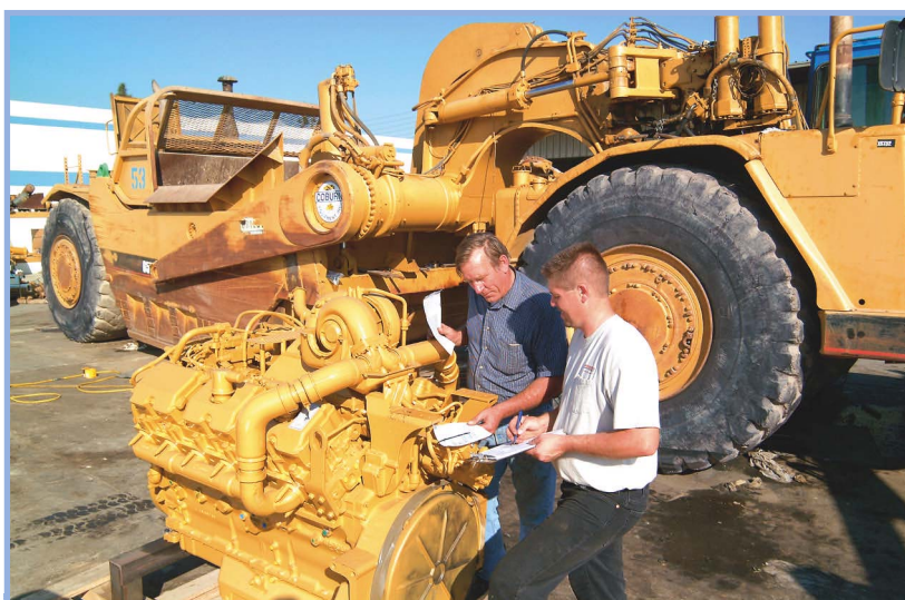
Ray Coburn (left) and equipment manager Mike Bowman take delivery of a new scraper engine. Coburn Equipment, a Chino, Calif., firm, is using Carl Moyer grants to repower tractors at the cost of rebuilding engines.
