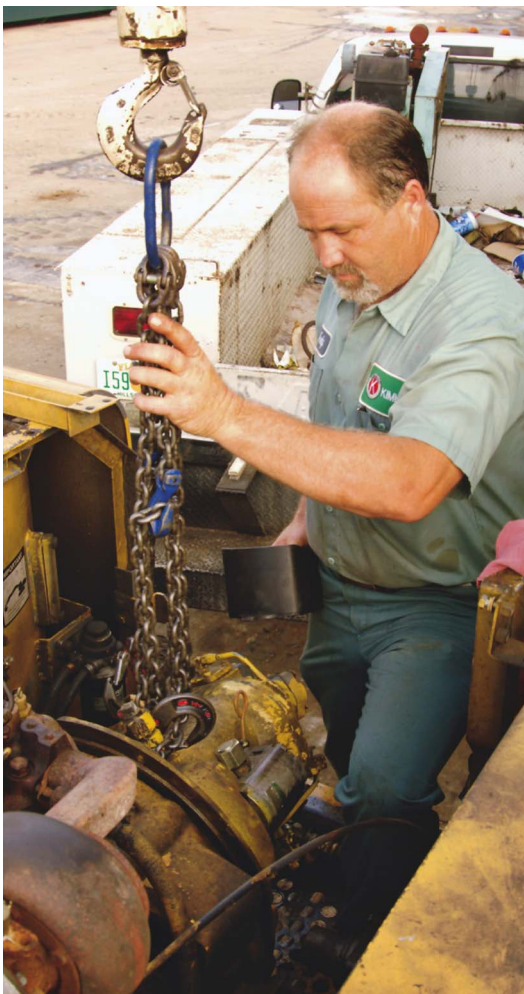
Jody Coombs, mechanic, changes the flywheel and ring gear on a John Deere 790 excavator's engine. Kimmins routinely keeps machines running out to 15,000 to 20,000 hours.
